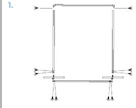
Layout poles in correct shape and screw in bolts to connect the polies together with the screws provided.
