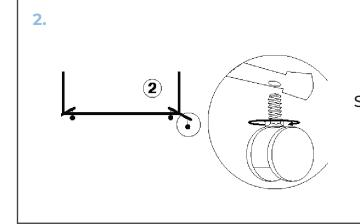
Screw in wheels to the bottom of frame.
